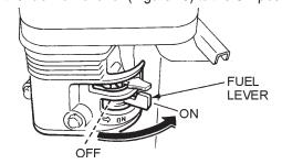
Figure 19. Engine Fuel Valve Lever
